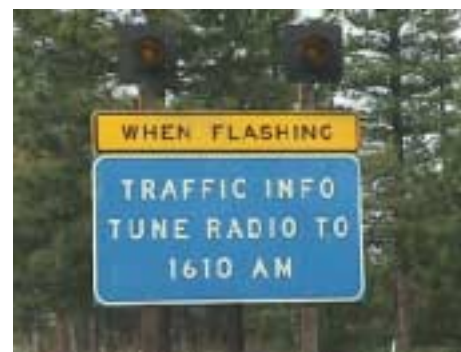
Figure 5-9: Example of Highway Advisory Radio Signage.
