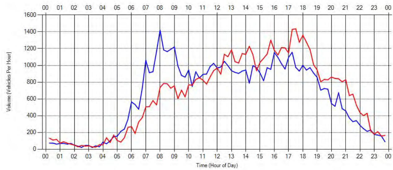
Approach Volume University Avenue @ East Bay Boulevard - SIG#6402 Wednesday, May 17, 2017 12:00 AM - Wednesday, May 17, 2017 11:59 PM Northbound and Southbound Approaches Wavetronix Matrix at stop bar
